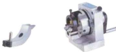
Shapes of punches formed by holding a punch on GIN - PFB and by Grinding on surface grinder.
